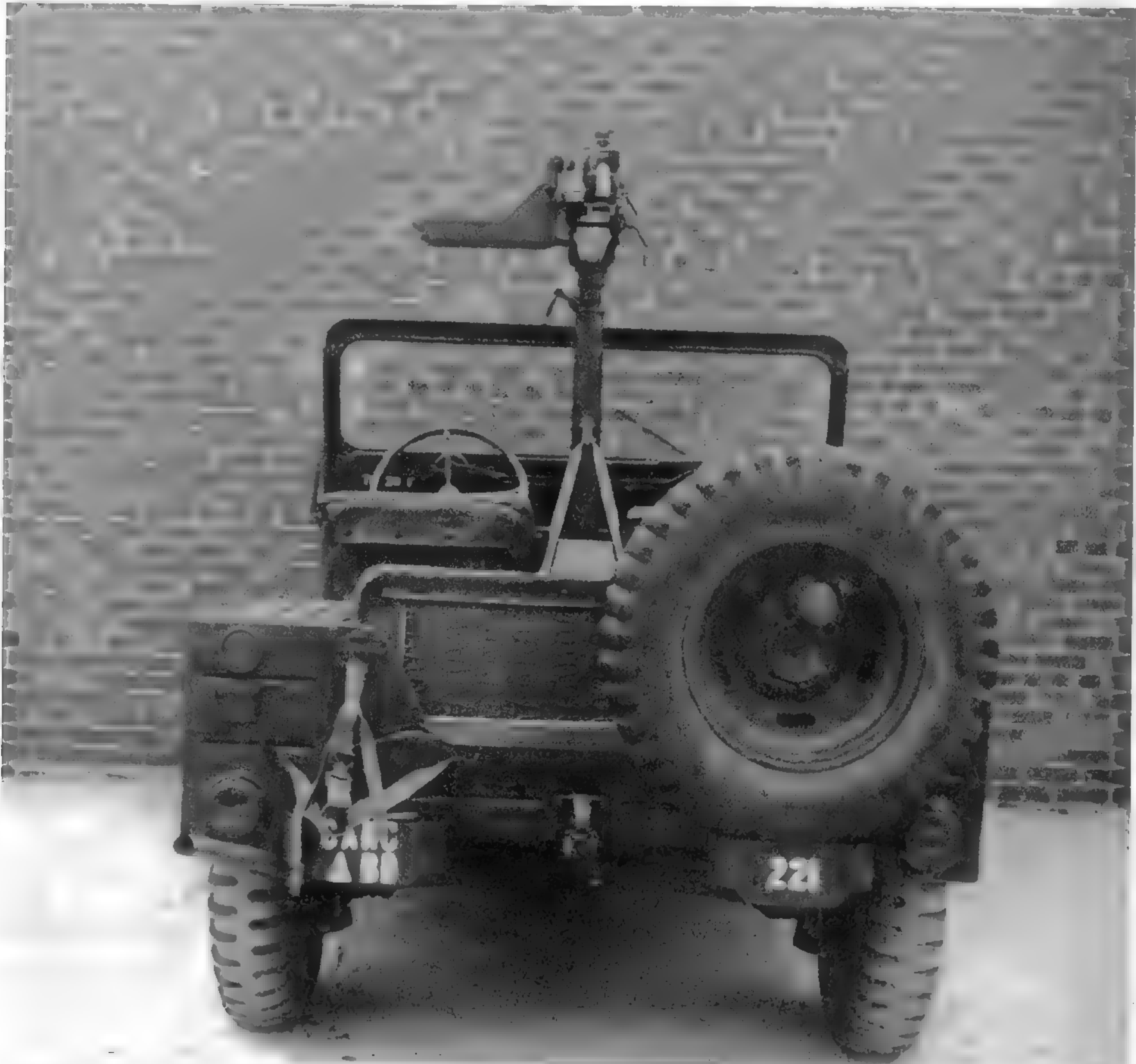
The M151 family did not use the traditional liquid container bracket. Instead, the spare gas can sat on the left bumperette, and was secured by a Y-shaped webbing strap. (Photo courtesy of the Patton Museum)
